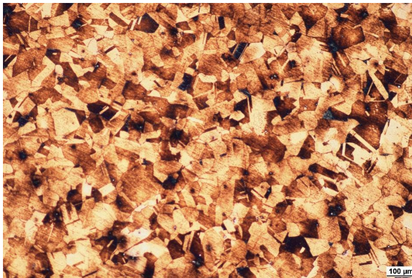
Figure 2 optical image of a blank 304 stainless steel specimen
