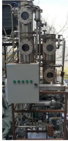
Figure 3 The experimental dual-functional AHE unit
