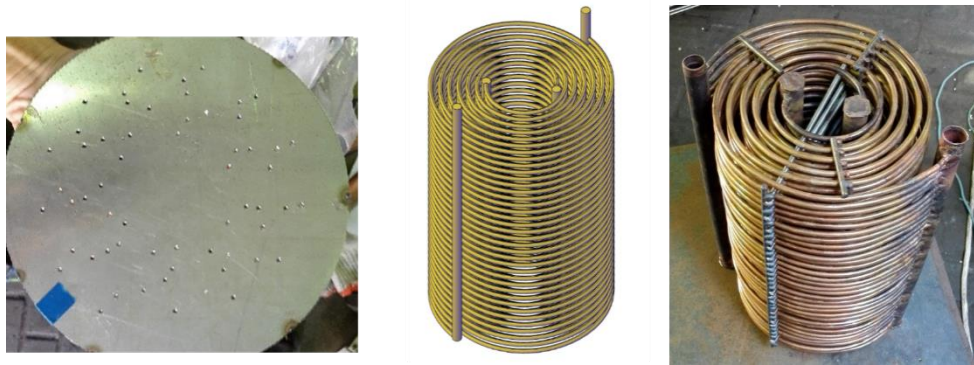
Figure 4 Internal components of the DFAHE: (a) copper coil assembly and (b) solution distribution plate
